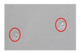
Significant differences in the melt behaviour of polymers combined during coextrusion will lead to sheets with bad surface quality.
