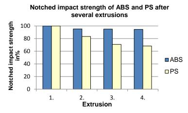
Under high temperatures all thermoplastic materials show a degradation of their molecule structure which means that depolymerisation takes place. While this degradation process may vary according to raw material grade or type, the result is a reduced molecule size that causes the loss of mechanic properties. Depending on the type of application it is advisable not to use 100% regrind during extrusion but to combine regrind with virgin material.
